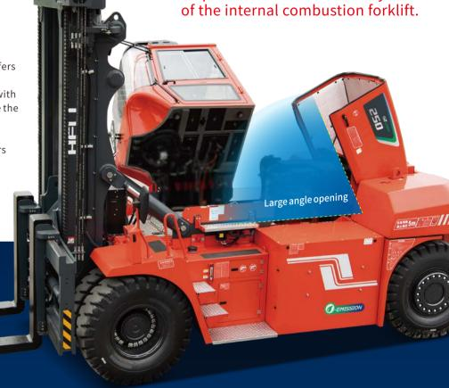
The truck is equipped with potential energy recovery and kinetic energy regenerative energy technology, thorugh which the energy is recovered and supplemented to the battery, further improving the system efficiency and truck life. The annual comprehensive use cost of electric truck is only 42.5% of the internal combustion truck.
